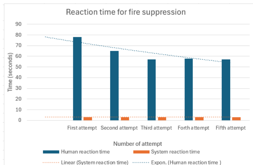
Figure 22: Reaction time for fire suppression
