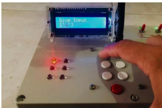
Figure 10: Braille Input and Display Output for Letter 'a'
