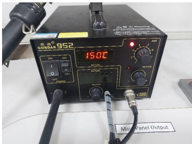
Figure 15: Using the hot air to simulate the high temperature
