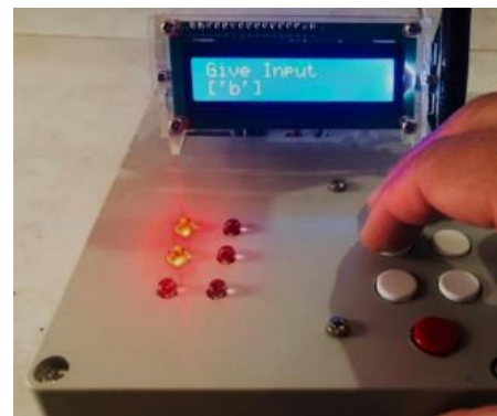
Figure 11: Braille Input and Display Output for Letter 'b'
