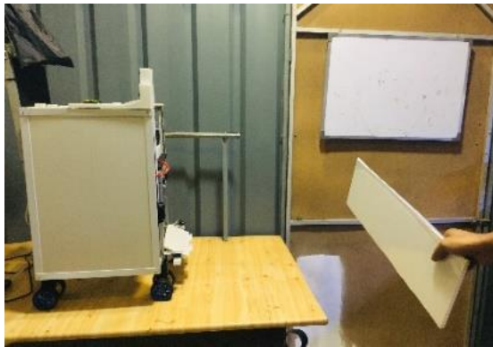
Figure 7: Ultrasonic sensor detecting distance testing
