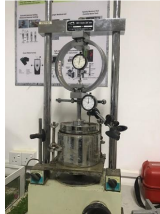
Figure 5: California bearing test
