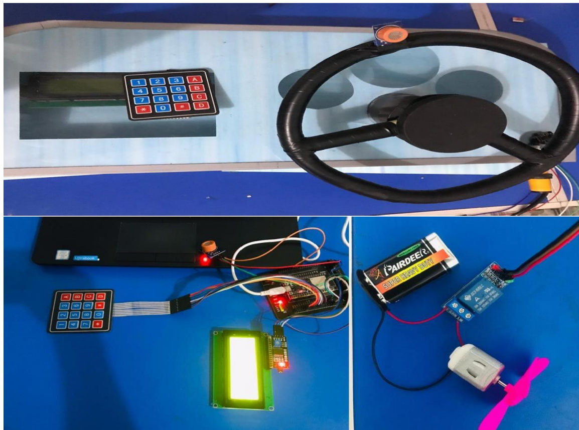
Figure 15: Prototype of Control System of Alcohol Based Vehicle Hazard
